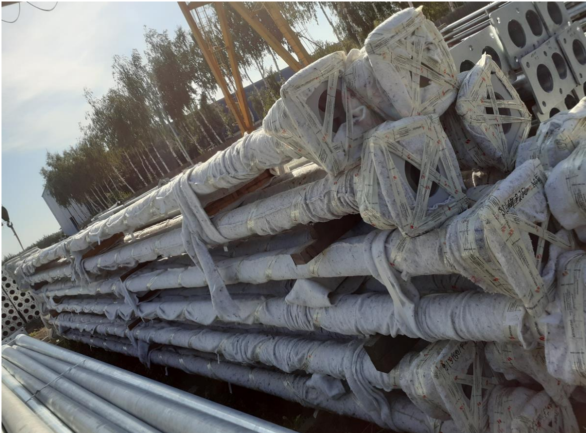
b) Packaging of poles covered with a paint system: - the poles should be packed in a cover along their entire length.
